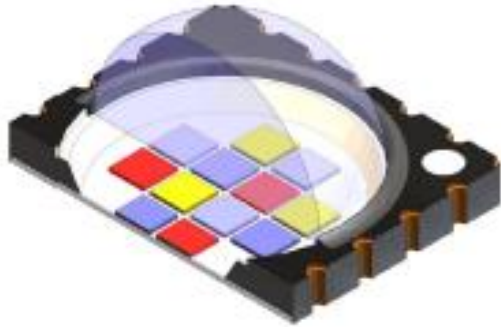
Fig. 1. LuxiGen™ emitter cross-section and customizable die combination in a LZC emitter
